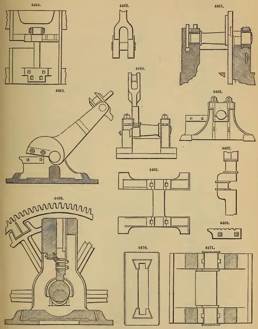
elevation and plan of framing for shears; Fig. 4467, shears-crank; Fig. 4468, knife for cutting bars; Figs. 4469 to 4471, cross-section, plan of frame, and sectional plan of an eccentric shears. The speed of the puddling rolls ranges from thirty-five to eighty revolutions a minute. The Staffordshire and Derbyshire forges probably work at the lowest speed of any in this country. The Welsh forges are driven from fifty to eighty. The speed preferred by the workmen, and which
